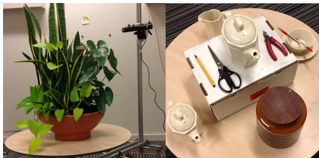
Figure 10. Two test scenes scanned by rotating a Kinect around the table as shown in the left figure. Vicon markers for ground truth tracking were attached to the body of the Kinect.
