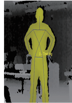
Fig. 2: Human skeleton model from the Kinect sensor.
