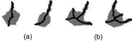
Fig. 16. Some confusing cases for skeleton matching [3], where very different shapes have similar skeletons.
