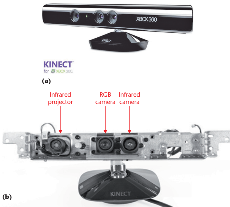
Figure 1. Microsoft Kinect sensor. (a) The Kinect sensor for Xbox 360. (b) The infrared (IR) projector, IR camera, and RGB camera inside a Kinect sensor.
