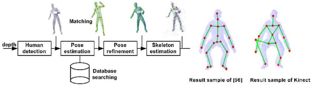
Fig. 8. Basic processing pipeline of algorithms reported in [56] and [57], where the image examples are from [56].
