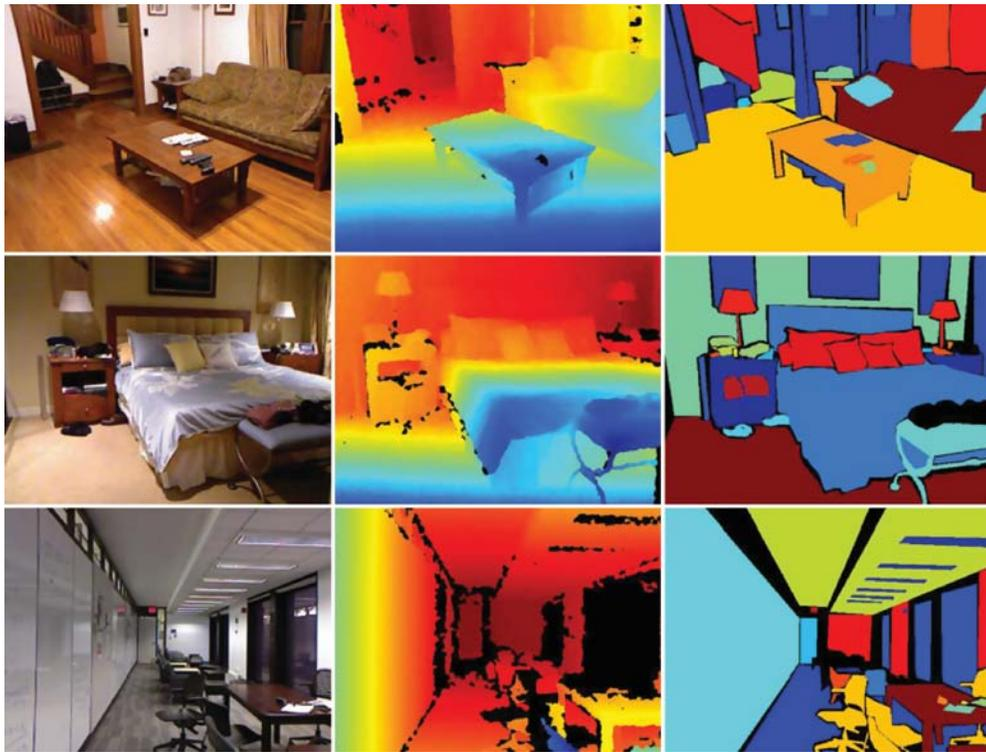
Fig. 7. Image samples from the dataset in [44]. From the left to the right: RGB images, depth images and annotated object regions with labels.
