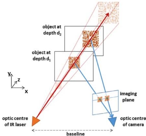
Fig. 3. Illustration of Kinect depth measurement.
