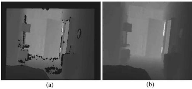
Fig. 4. Example for hole-filling based on the bilateral filter [25]. (a) Raw depth image. (b) Depth image after filtering.
