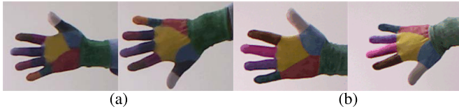
Fig. 2. Color glove design. (a) 14 and (b) nine patches.
