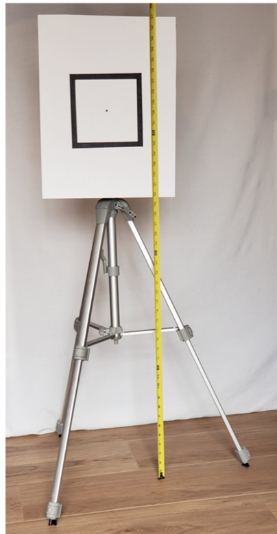
Figure 2. A planar board marked with a rectangle and a point is used as the test object for scanning.
