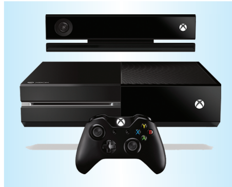
Figure 1. Xbox One Kinect, console, and wireless controller. The system recognizes individual users, who can use voice and movement to switch between functions; users can also interact with friends through various services, including Skype.
