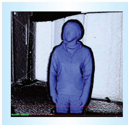
Figure 9. Depth image captured at a distance of 2.5 meters. The fine detail of facial features and folds in the clothing are clearly visible.
